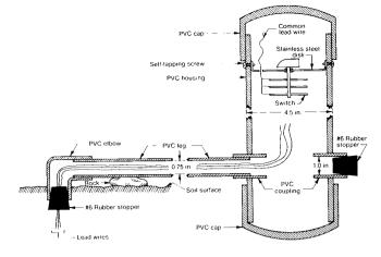
Fig. 2. Schematic of the spider housing showing leg attachment to housing, sealed coupling for an additional leg, and the position of the caps. Also illustrated is the distal end of the spider leg showing the attached elbow fitting and the rubber stopper which provides a seal around the lead wires. Small rocks are used to elevate each leg slightly above the soil surface.
