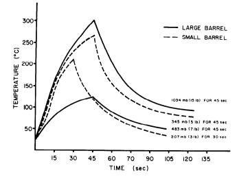
Fig. 3. Examples of time-temperature curves generated by various combinations of propane pressure and burn time for the large (107 cm) and small (58 cm) burn barrels.
