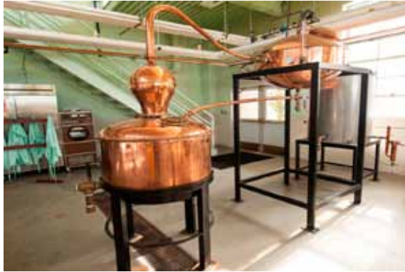
80 Gallon Alembic Pot Still donated by King Estate Winery Photo: Lynn Ketchum, OSU
